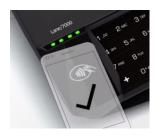
Your contactless terminal provides four contactless status lights located above the contactless logo.
