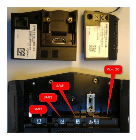
Insert the SAM Card into the slot marked (1), (2) or (3). Take care to ensure that the SAM
